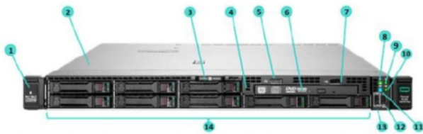
8 SFF Front View - 8 SFF + optional Universal Media Bay, optical drive, and SAS drives shown
